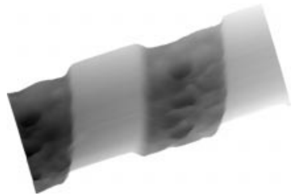
Figure 8: AFM surface image of source-drain and channels regions in an N-channel MOSFET.
