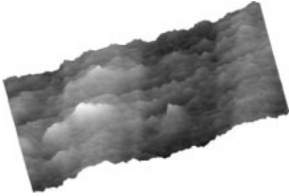
Figure 9: SKPM image of source-drain and channels regions in an N-channel MOSFET. Note the clear delineation of the change from the heavily-doped to the lightly-doped region.
