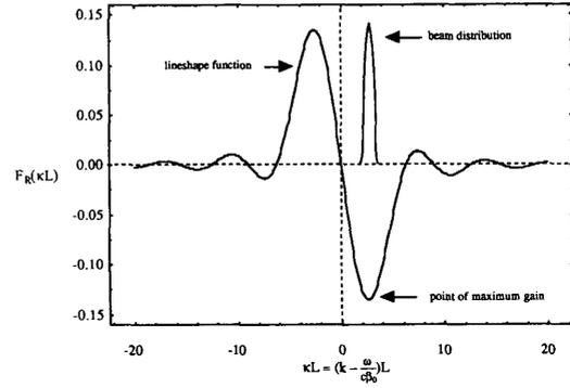
Fig. 4. The single particle line shape function is plotted versus phase mismatch,  $\kappa L$ . An approximately monoenergetic beam distribution is also shown to illustrate the permissible degree of phase spread.
