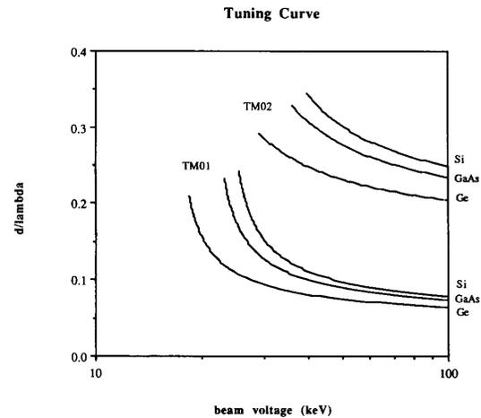
Fig. 3. The tuning curve is shown for the lowest order TM modes of Si, GaAs, and Ge. This plot of dielectric thickness-output wavelength versus beam voltage is generated from the dispersion relation by imposing the synchronism condition.
