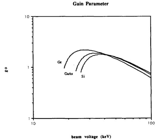
Fig. 5. The gain parameter  $-g_o$ , is plotted versus beam energy for the  $TM_{01}$  mode of Si, GaAs, and Ge. The second branch solutions are larger by a barely discernible amount on this scale.
