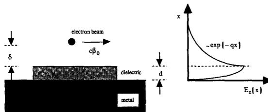
Fig. 1. The Cerenkov laser mechanism is shown schematically. An electron passes a distance  $\delta$  from a thin dielectric slab. The  $z$  component of the electric field to which it couples is also shown.
