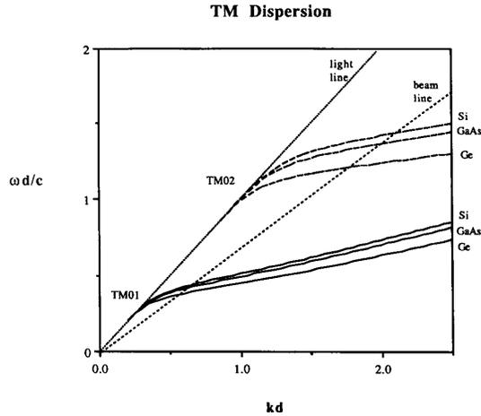
Fig. 2. The  $TM_{01}$  and  $TM_{02}$  solutions to  $D(\omega d/c, kd, \epsilon) = 0$  are shown for the three dielectric constants corresponding to Si, GaAs, and Ge. The light line and beam lines indicate the phase velocity of the light in vacuum and the beam velocity, respectively. Synchronism occurs at intersections of the beam line and the dispersion relation.
