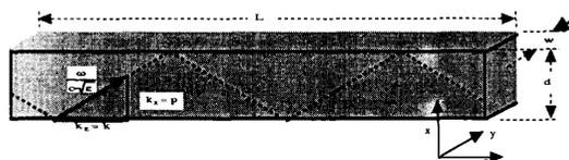
Fig. 6. A schematic of the dielectric film dimensions and coordinate system. The ray optic view of wave propagation is illustrated with the wave-number decomposed into  $x$  and  $z$  components.
