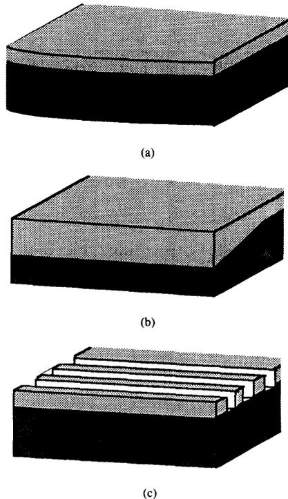
Fig. 7. Three possible mirror designs are shown schematically. (a) Slight curvature is introduced to match the Gaussian-mode wavefront and improve transverse confinement. (b) Adiabatic confinement of the evanescent mode ensures that the end mirrors reflect the entire mode. (c) The square profile distributed Bragg reflector is illustrated. Alternate cross sections and varying index materials exhibit similar pass and stopbands which can be employed as a reflector.
