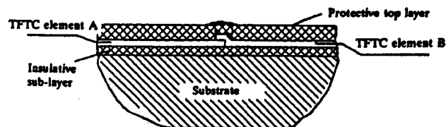
Fig. 1(b)—Schematic cross-section of thin film thermocouple.
